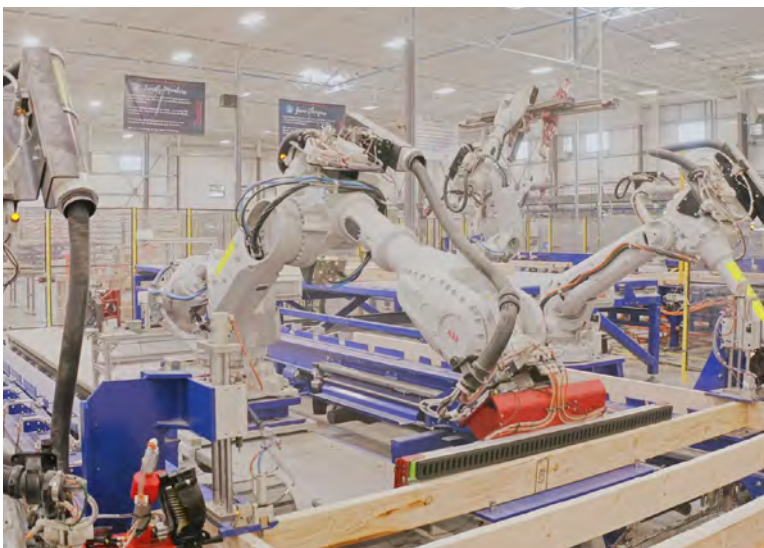
Floors, ceilings, and walls are assembled by robots—reducing physical stress and increasing precision.
