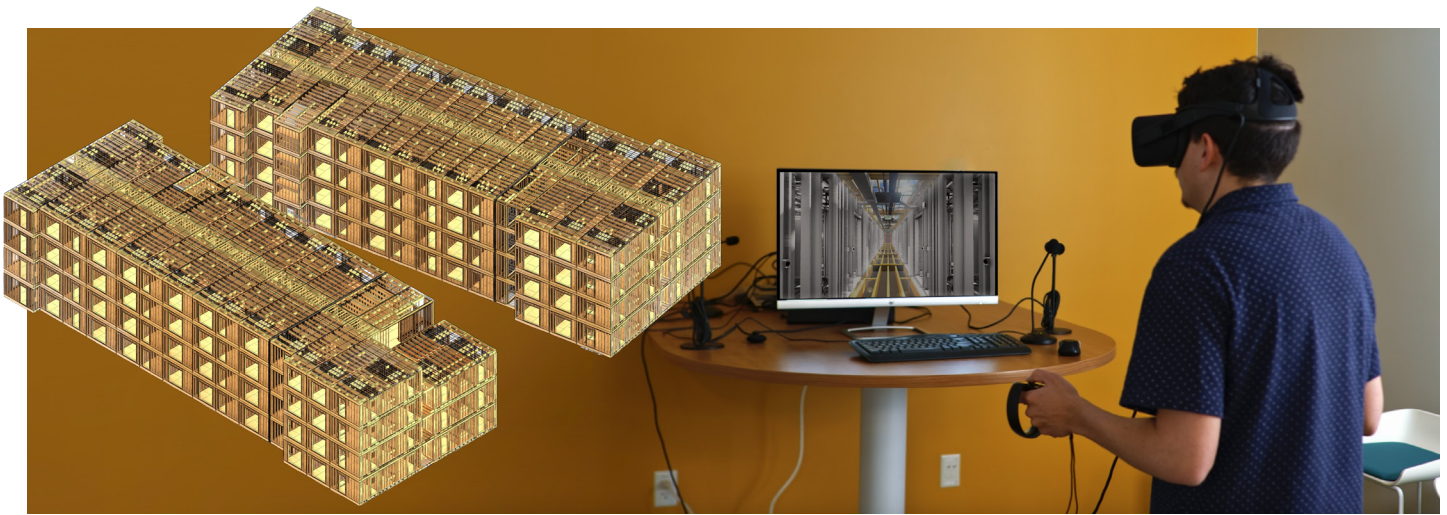
A digital twin of Sango Court provided data for VR reviews, clash detection, automation code, and AR models to guide factory and onsite tradespeople.
