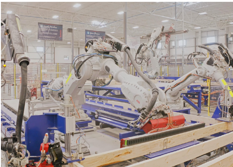
Floors, ceilings, and walls are assembled by robots—reducing physical stress and increasing precision.
